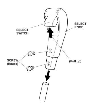
3. Reinstall the two screws.
