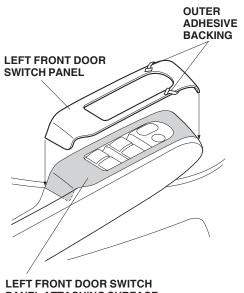
PANEL ATTACHING SURFACE (Clean with isopropyl alcohol.)
