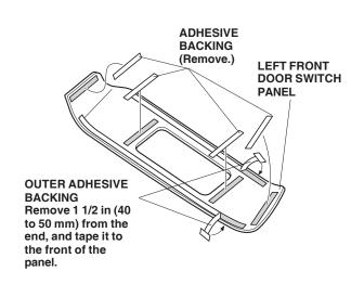
Remove and discard the inner adhesive backings and the small pieces of outer adhesive backings. Attach a strip of masking tape to the end of each remaining outer adhesive backing, and remove 1 1/2 in (40 to 50 mm) of the adhesive backing. Fold the ends back, and tape them to the front of the panel.
