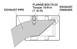
Start the engine, and rev it up a few times. Listen for vibration from the exhaust finisher, and adjust if necessary.
