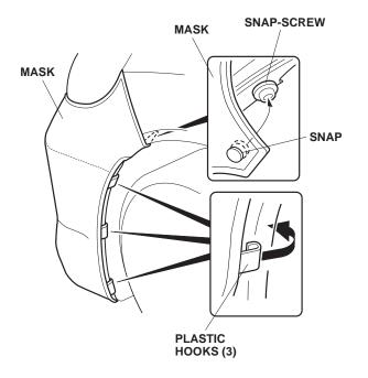
9. Repeat steps 7 and 8 to install the mask on the right side of the vehicle.
