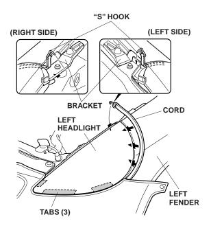
8. Pull the mask back toward the wheelwell, smooth out any wrinkles, and snap the mask to the snapscrew. Attach the three plastic hooks to the fenderwell.
