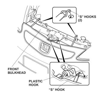
11. Attach the four hooks to the grille opening. Insert the two tabs between the grille and the front bumper, and attach the four plastic hooks to the bottom edges of the front grille.
