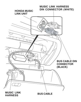
NOTE: To unplug the BUS cable DIN connector pull back on the lock release slide collar.
