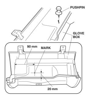
16. While wearing eye protection, drill a 19 mm hole through the glove box at the marked location. First drill with a 3 mm drill bit wrapped with electrical tape 30 mm from the tip, and finish with a 19 mm hole saw.
