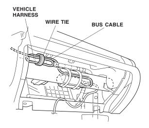
30. Secure the Music Link harness to the vehicle harness with one wire tie at the location marked in step 18.
