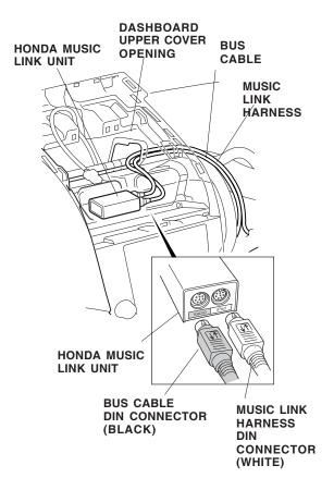
25. Mount the Honda Music Link unit behind the steering hanger beam with the two long wire ties.
