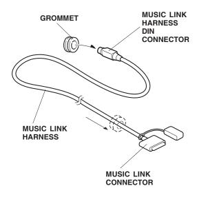
18. Using felt-tip pen, mark the Music Link harness at the measurement shown.
