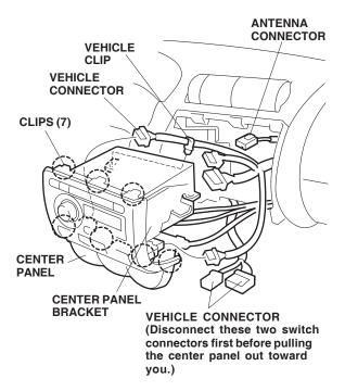
14. Unplug the vehicle connectors, and the antenna connector from the center panel unit, and remove the center panel (on some models, it is necessary to release the vehicle harness clip from the hole in the center panel bracket).
