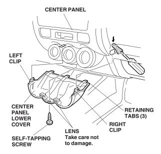
7. Reach through the center panel lower cover opening and remove the two screws that secure the center panel bracket.
