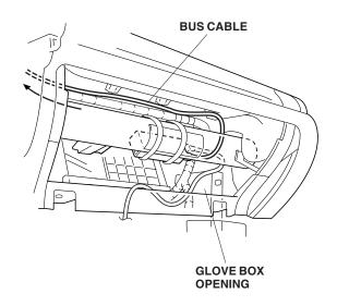
27. Align the BUS cable 14-pin connector with vehicle connectors, then secure the BUS cable to the vehicle harness with one wire tie.
