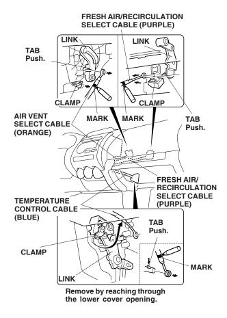
12. Using a felt-tip pen, mark the location of the TEMPERATURE CONTROL CABLE at the clamp. Remove the TEMPERATURE CONTROL CABLE from the clamp, then push down on the tab and slide the cable from the link pin. Take care not to damage the pin and mounting seat of the clamp when removing the cable.  Pull the center panel out toward you (seven clips).
