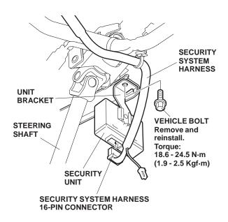
18. Plug the security system harness 16-pin connector into the security unit.
