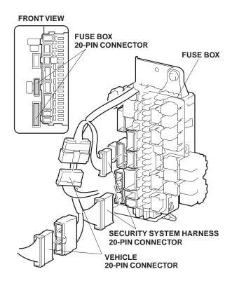
12. Remove the dummy connector from the keyless entry harness.
