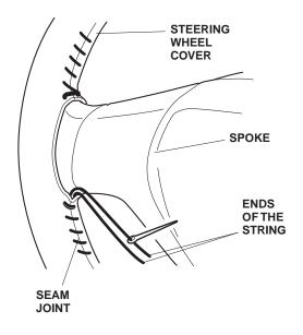
14. After installing the steering wheel cover, use the palm of your hands to hold pressure against each section for 30 seconds to secure the adhesive.
