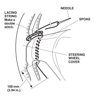
Pull the string from the double-stitched lacing hole on the back to the next lacing hole on the cover.
