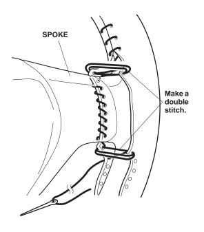
13. When lacing has been completed, pull the string out of the cover opening. (Confirm that both ends of the string come out at the seam joint of the cover.) Tie a tight double knot, and cut off the excess string at the knot. Hide the knot by pushing it into the inside of the steering wheel cover.
