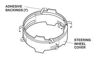
2. Place the steering wheel cover over the steering wheel with the nonholed sections of the wheel cover aligned with the spokes of the steering wheel as shown.
