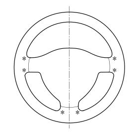
10. Continue lacing so that the two edges of the cover are aligned along the inner radius of the steering wheel.
